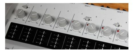
The knobs pictured at left are the input volume control knobs, beneath which are the volume indicator lights, which light up green, orange, and red as your levels approach clipping. Your input source volume should not exceed -6dB.
