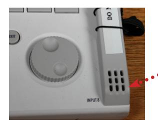
Built-in microphones are located on either side of the R16, in the corners, marked as inputs 7 and 8.
