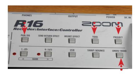
The buttons at left toggle the R16's menus. The most important buttons on this panel are PAN/EQ, TOOL, PROJECT, and and UNDO/REDO
